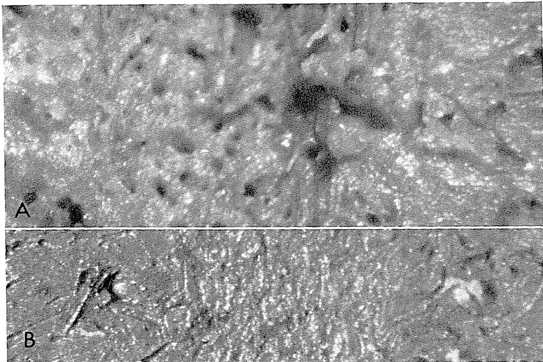
FIG. 3a. Deformation of clay slope showing fine detail;  $e_w = 1.3$  ( $\times 100$ ).
