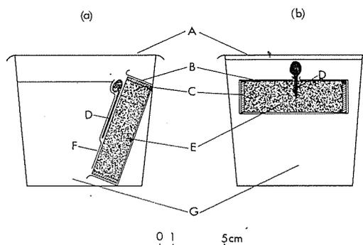
FIG. 1. Assemblies used to grow radicles (a) down clay slopes, (b) through clay cores. A polyethylene film; B aluminum foil; C consolidometer ring; D radicle; E clay core; F polyethylene diaphragm; and G wet sand.
